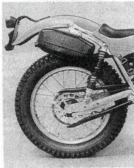
The Cota features Betor shocks. The enclosed chain shield is unique to Montesa.
