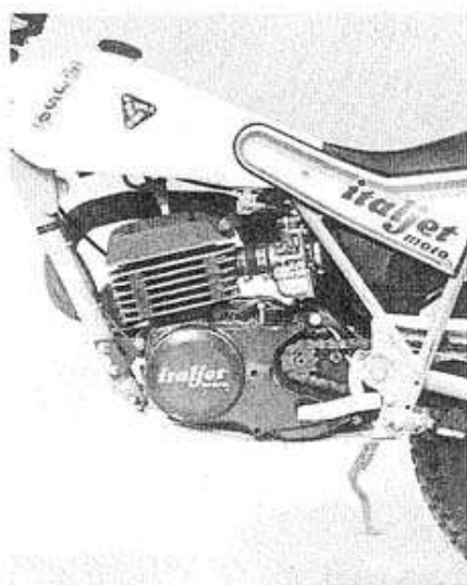
Italjet's 350T has a 83.2 x 60mm bore and stroke. A 28mm Dell'Orto mixes the fuel.
