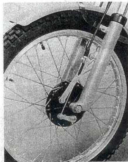
Montesa makes their own fork. Distance between the fork legs was widened for 1983.
