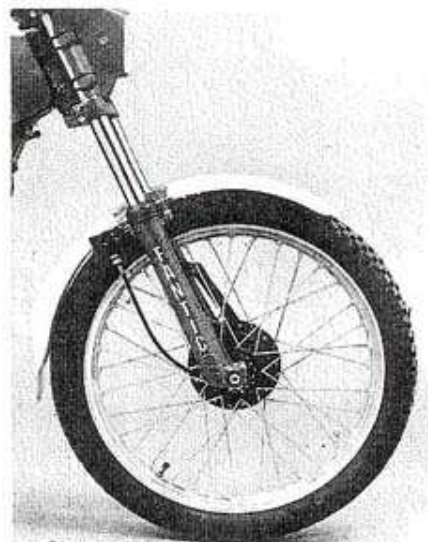
Leading axle fork on the Fantic is manufactured by Marzocchi.
