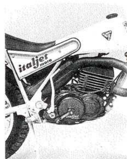
The right-side shifter shown on the Italjet is available as an accessory option.
