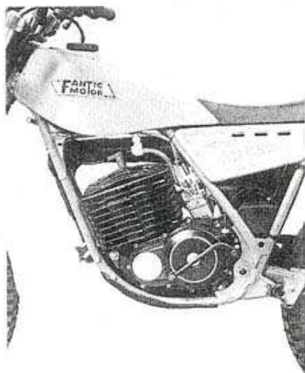
Fantic's 212cc motor produces exceptional power for its size. Compression is 11.7:1.
