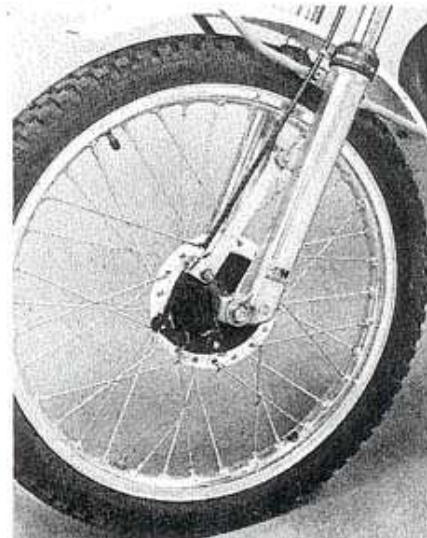
The Italjet 350T has a 35mm Marzocchi fork. The Pirelli tires are standard equipment.
