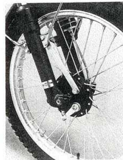
The Cagiva's fork is made by Betor. All five bikes use Akront aluminum rims.
